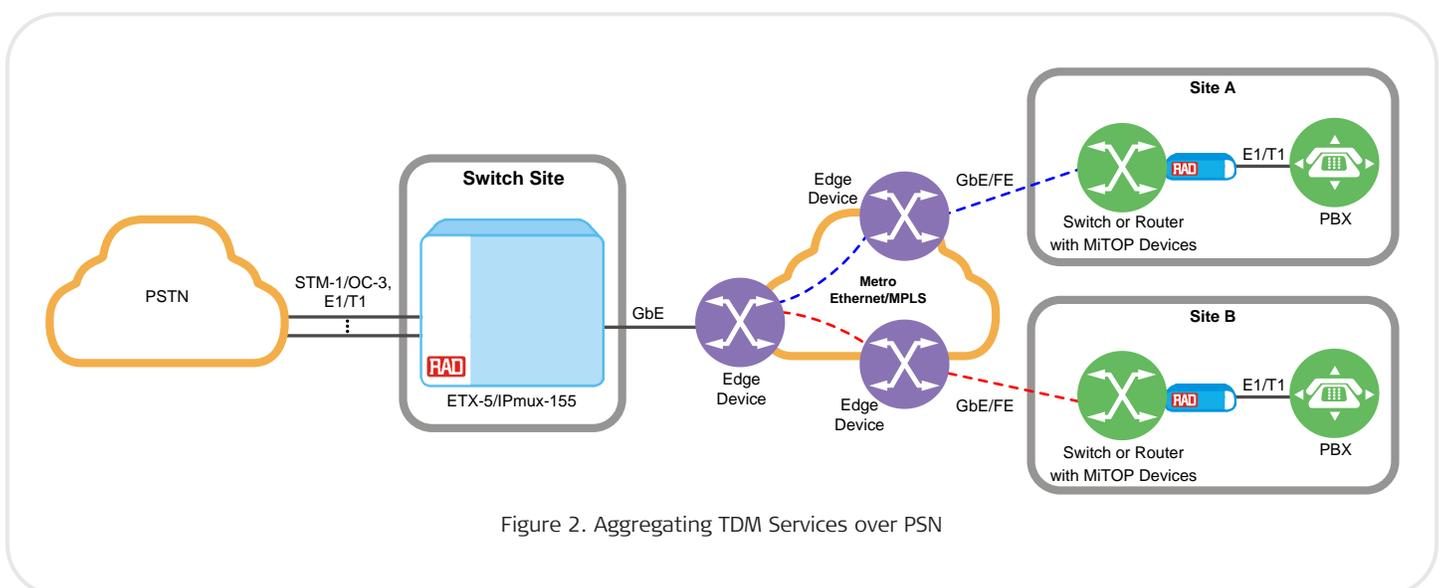
Figure 2. Aggregating TDM Services over PSN
