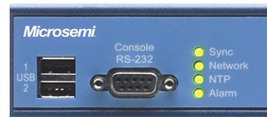
Informative Status LEDs provide at-a-glance health of the network time server. The USB ports add additional flexibility in back-up, restore and upgrade operations.
