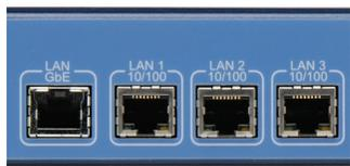
Four network ports (including Gigabit) provide network configuration flexibility and enhanced security. "Multiple" isolated and synchronized time servers can also be configured.
