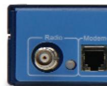
Internal modem and optional AM radio antenna provide access to national time sources for time reference redundancy.
