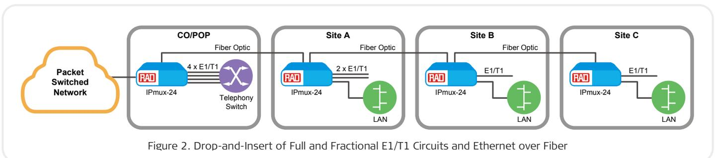
Figure 2. Drop-and-Insert of Full and Fractional E1/T1 Circuits and Ethernet over Fiber
