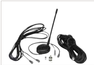
GMAE4290 Combined TETRA and GPS antenna for digital car kit operating in the 380-430MHz frequency range - includes duplexer and DC adapter. Compatible with car kits GMLN4687 and GMLN5076.
