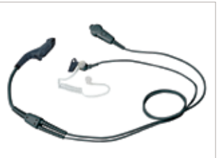
RLN5882 2-wire receive and transmit surveillance kit in black with acoustic tube and one programmable button.
