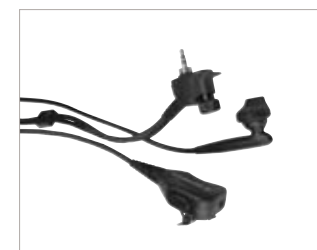
FTN6707 2-wire surveillance kit in black with combined microphone and push-to-talk.
