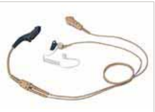
RLN5883 2-wire receive and transmit surveillance kit in beige with acoustic tube in-line PTT and one programmable button.
